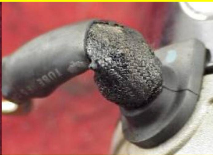
Motor strap insulator discolored by over-crank.
